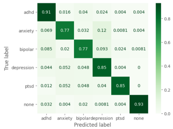
Fig. 25. Normalized Confusion Matrix for Mental Illness generated after classifying the test dataset using the trained BERT model with a dropout of 0.15
